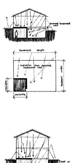
If it is found to be impractical to shield one quarter of the basement ceiling area, the extent of ceiling modification may be reduced to any desired size by constructing vertical masonry walls on the two open sides of the shielded area, thus providing a room suitable for use as a hobby or laundry room. These masonry walls will also provide protection from excessive amounts of radiation coming through exposed portions of the basement wall.
