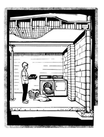
Protection is provided in a basement corner by bricks or concrete blocks between the overhead joists. A beam and jack column support the extra weight.
