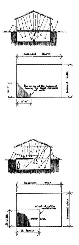
This cross-section of a one story house shows radiation coming into the basement from fallout particles on the roof and the ground, Most of the radiation comes from the roof because of the shielding effect of the ground outside the basement walls.
